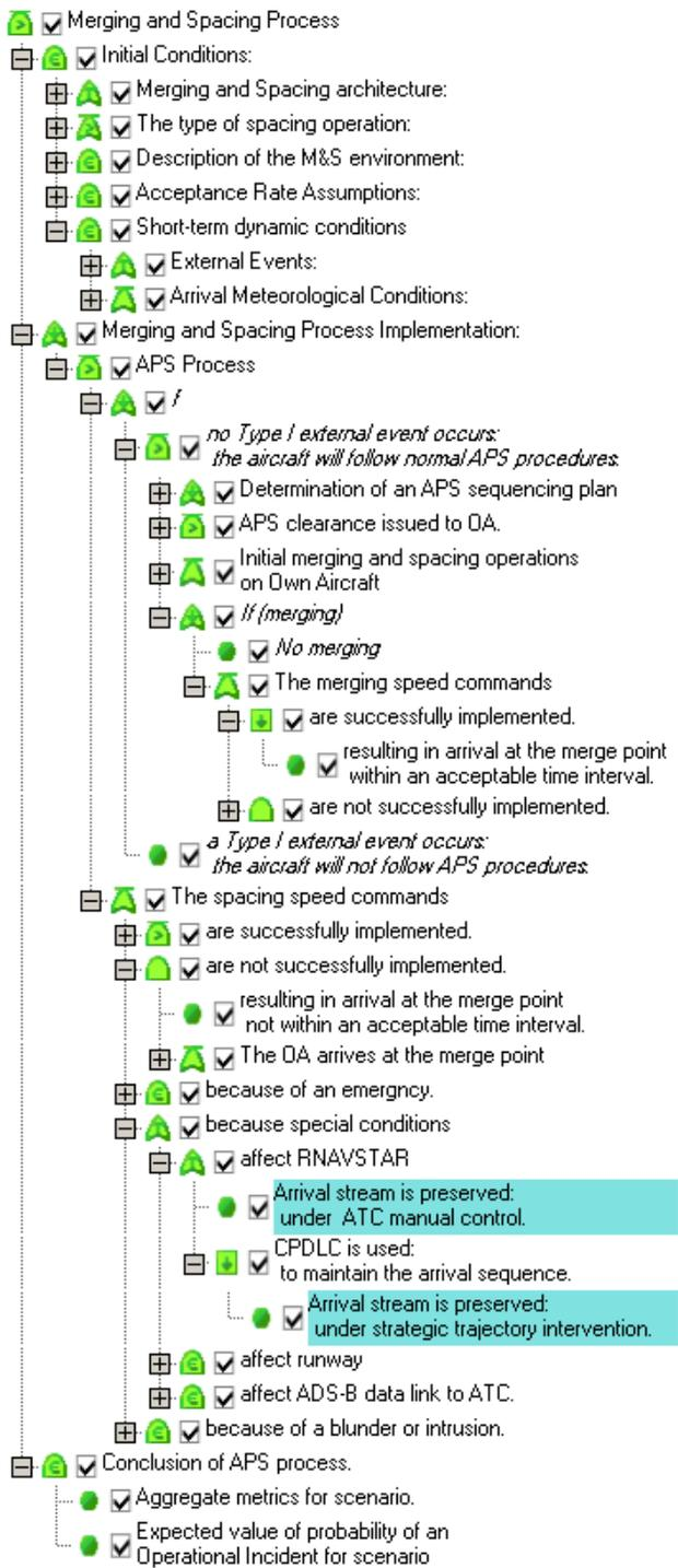
Figure 3. Translation of APS block diagram to an LGM
