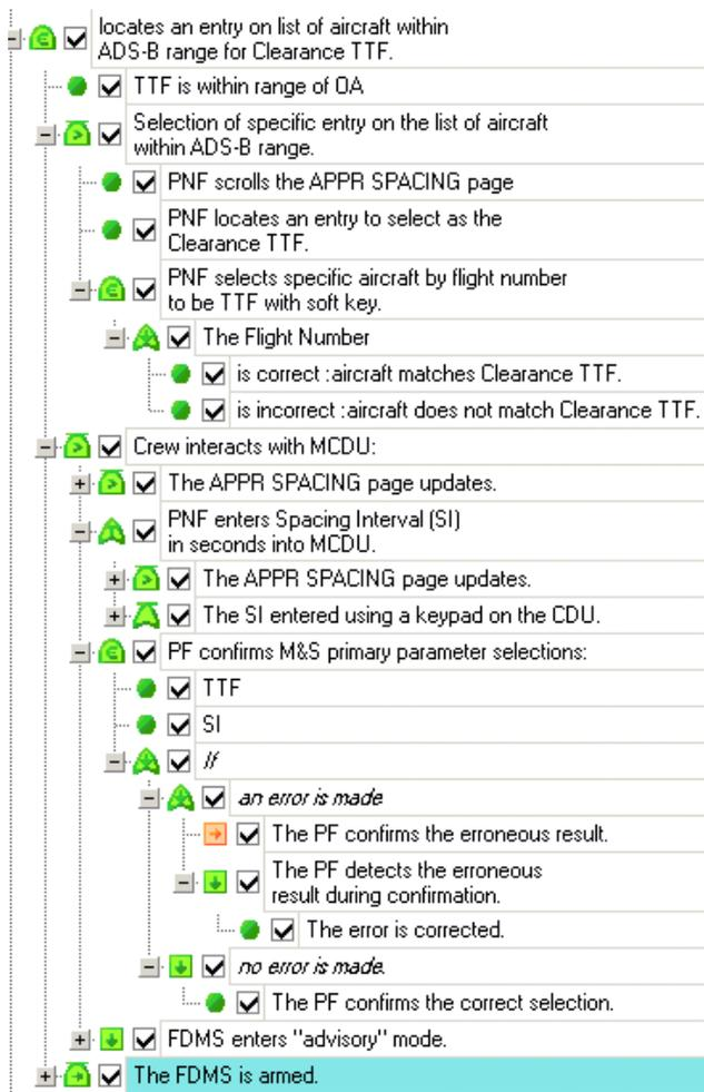
Figure 4. Sub-model for APS setup showing the start of an incident sequence
