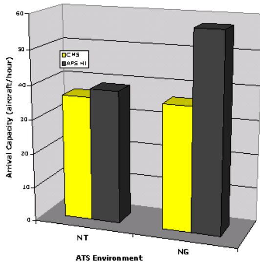
Figure 7. Arrival Capacity for CMS and APS for Near-term and NextGen Demand States
